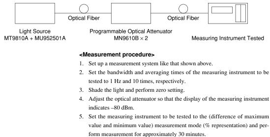
6. The noise level can be calculated from the following formula, using the measured value when the measurement is completed.
